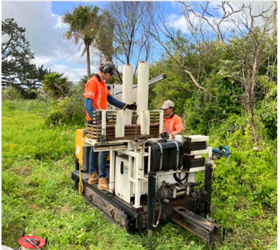
Above: core drilling near Flyers Road on the Marsden Point Rail Link route, to understand the geology. Below: ground testing at Oakleigh
