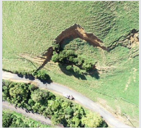
Rail line north of Tahekeroa, at the base of a large slip. We need to understand what is happening below ground.
