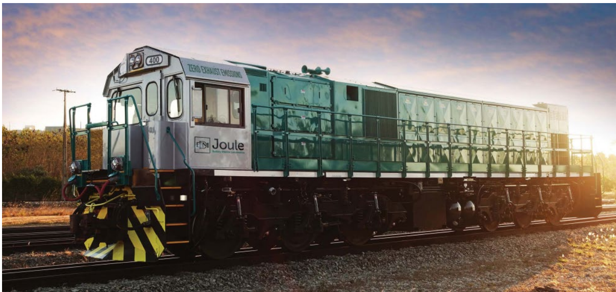
Figure 41: EMD (Progress Rail) GT38J 1.5-2.1 MW / 4.0 MWh "Joule" battery electric locomotive
