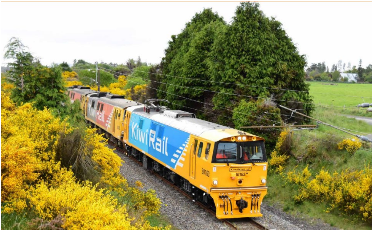
Figure 14: KiwiRail has current experience with Overhead Line Electrification and electric freight locomotives. This train shows the lead refurbished EF class electric locomotive on one of its early tests in December 2022. It is towing unrefurbished EF locomotives as part of the test load.
