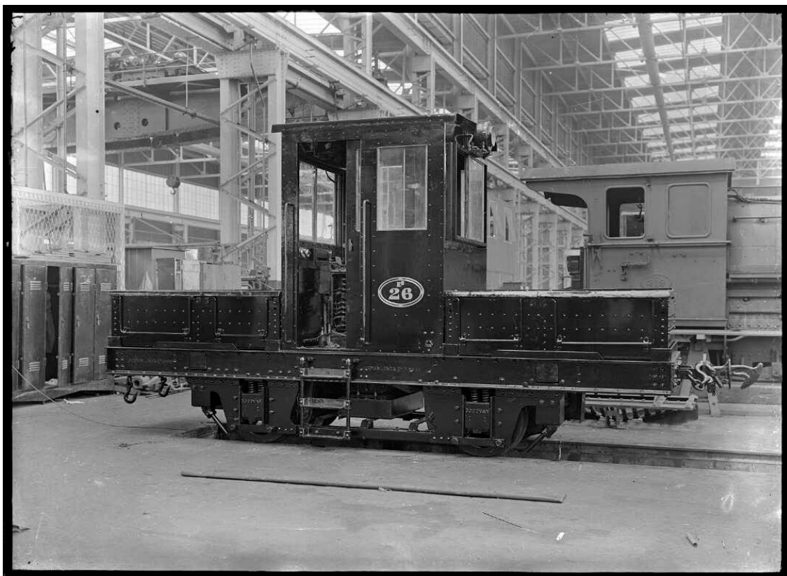
Figure 43: Battery shunt locomotives are not new. NZR Eb class battery – electric shunting locomotive (fleet entered service 1925 and 1929). Considering the subject of this report, it is perhaps ironic that this class of five battery locomotives were converted to diesel-electric from 1953, running as diesel locomotives until the end of their lives. 108
