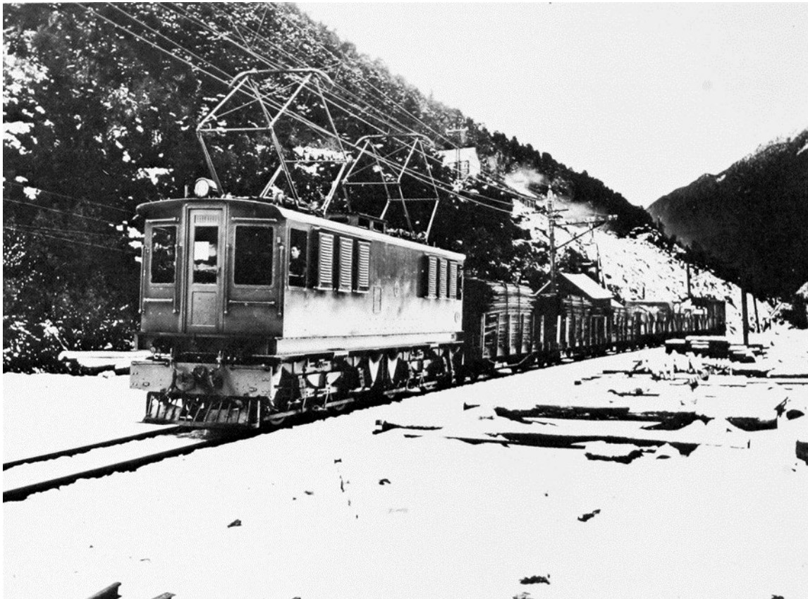
Figure 13: Railways in New Zealand have experience with operating overhead line electrification going back 100 years. First generation 1500 volt DC electric locomotive at opening of Oira-Arthurs Pass section in 1923.
