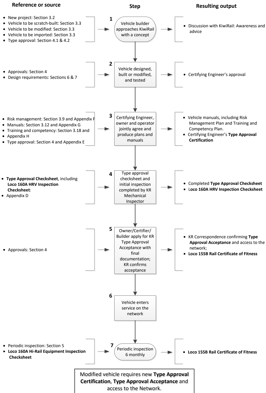
Figure 1: Process for scratchbuilt, modified or imported vehicle.
