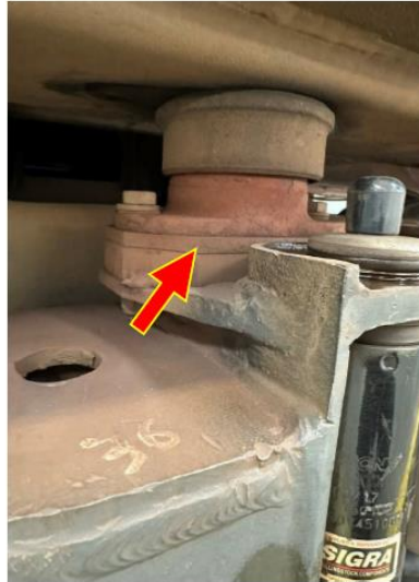
Red-coloured side bearers being found across the fleet. The red is indicative of iron fretting
