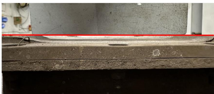
Worn wear liners with a very rough finish. Normally they are smooth and evenly worn
