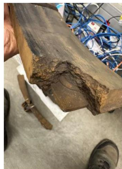
Brake blocks from myriad carriages; the failure mode is new
